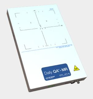
The Daily QA-MR enables efficient routine QA with single beam measurement results for Energy, Output, Transverse, Axial Symmetry, Shape Constancy, and Field Size Shifts (FFF). Accepted data is automatically written to a database in real-time, and is immediately available for trending, review and analysis.
